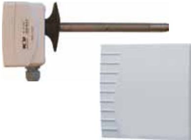
Room / Duct hygrometer for registration of the air humidity Switching capacity 24 - 250 VAC 2A Setting range 35 - 100 % r. F Protection class IP 30 / 65
