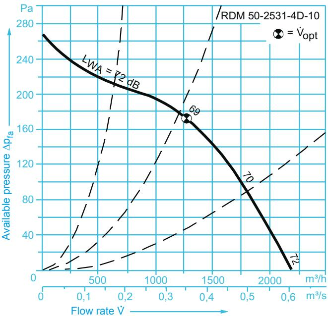
In the curves the A-weighted sound power level is  $L_{WA}$  ( $=L_{WA3} - L_{WA8}$ ) acc. to DIN 45635-38.
