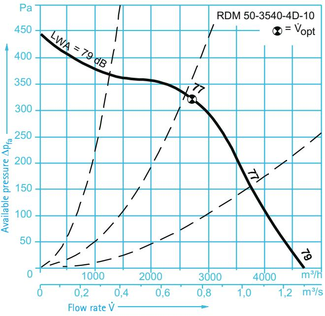
In the curves the A-weighted sound power level is  $L_{WA}$  ( $=L_{WA3}=L_{WA8}$ ) acc. to DIN 45635-38. Reference media density:  $\rho_1 = 1.15 \text{ kg/m}^3$ .
