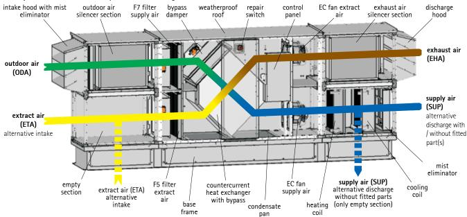
**Note:** Extract air intake and supply air outlet can be arranged as required, horizontally or vertically. Please note that a horizontal arrangement of the supply air outlet is only possible when there are fitted parts like heating or cooling coil and mist eliminator downstream the supply air fan.
