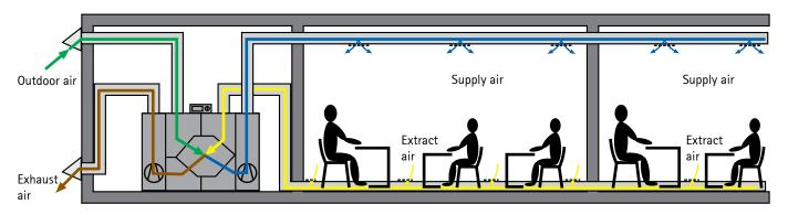
Minimum clearance between outdoor air intake and exhaust air discharge to prevent an "air short circuit" (DIN EN 13779)
