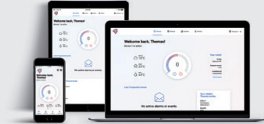
**Thermia Online** is a service that enables heat pump operation to be controlled from any location by means of any smartphone, computer or tablet with Internet access.
