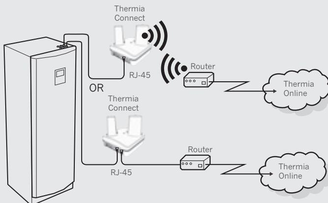
Thermia Connect is required for Legend, Legend Duo, iTec XT, iTec Eco. Thermia Connect can be connected to the router wirelessly or via an Ethernet cable (RJ45 connector).
