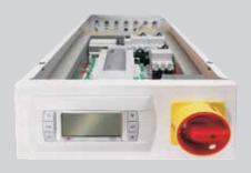
The microprocessor-controlled control unit, with an isolator on the appliance, is fully assembled and wired at the factory. It controls and regulates the fans, heat recovery, temperatures, flow rates and operating times, as well as a variety of internal functions and alarms.
