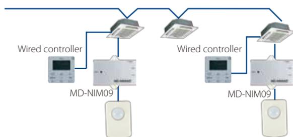
Remote controller or wired controller can control indoor unit.
