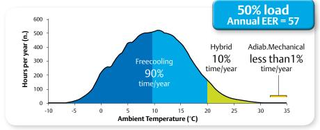
The above graphs and values refer to an application in London with 30% glycol mixture and inlet-outlet liquid temperatures of  $26^{\circ}-20^{\circ}$ C.
