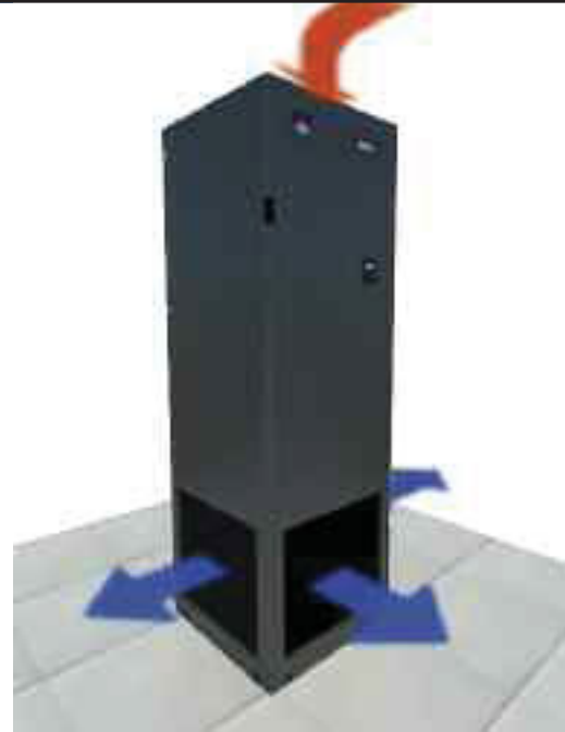
floor level (displacement) air delivery
