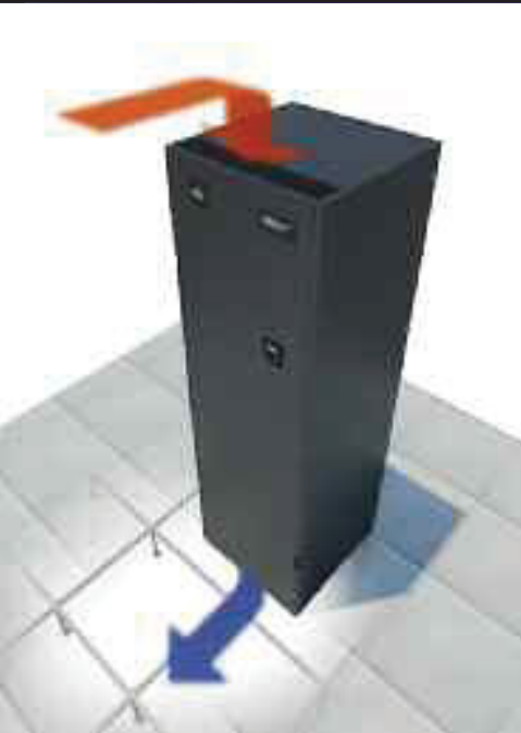
under floor air delivery
