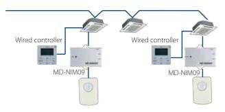
Remote controller or wired controller can control indoor unit.
