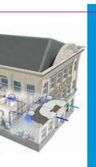
You can use the decorative elements on a building's façade, such as pediments or logos, to hide the grilles making the installation completely invisible
