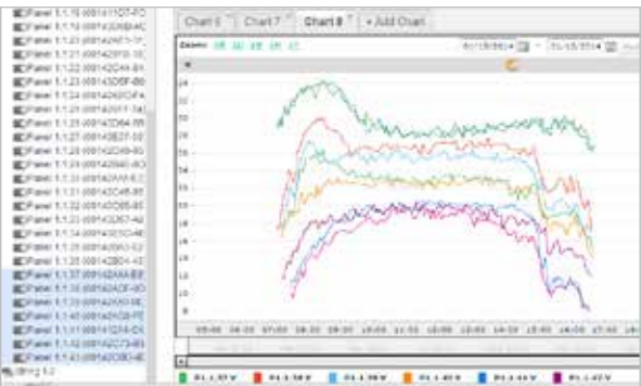
No need to send technicians to the roof – module voltage is measured remotely
